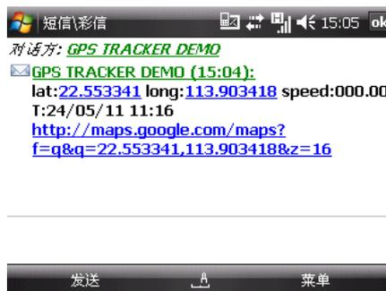
5.7.3 When lost fix to satellites, it will track by LBS / CELL-ID. And the SMS will include two positions:
